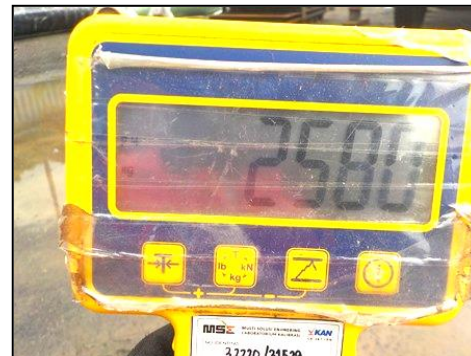
Figure 2. Reading actual Load test 2,500 Kg on digital load monitor.
